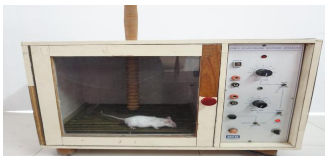
Fig. 3. Cook's pole climbing apparatus
