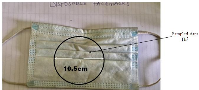
Fig. 7. Picture of Disposable face mask (inner surface) showing diameter of sampled area
