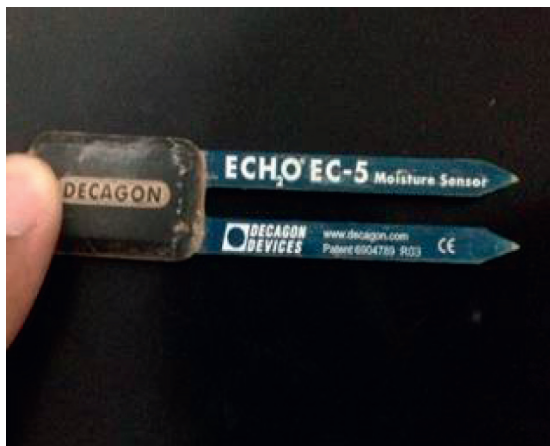
FIGURE 4: EC-5 soil moisture sensors.
