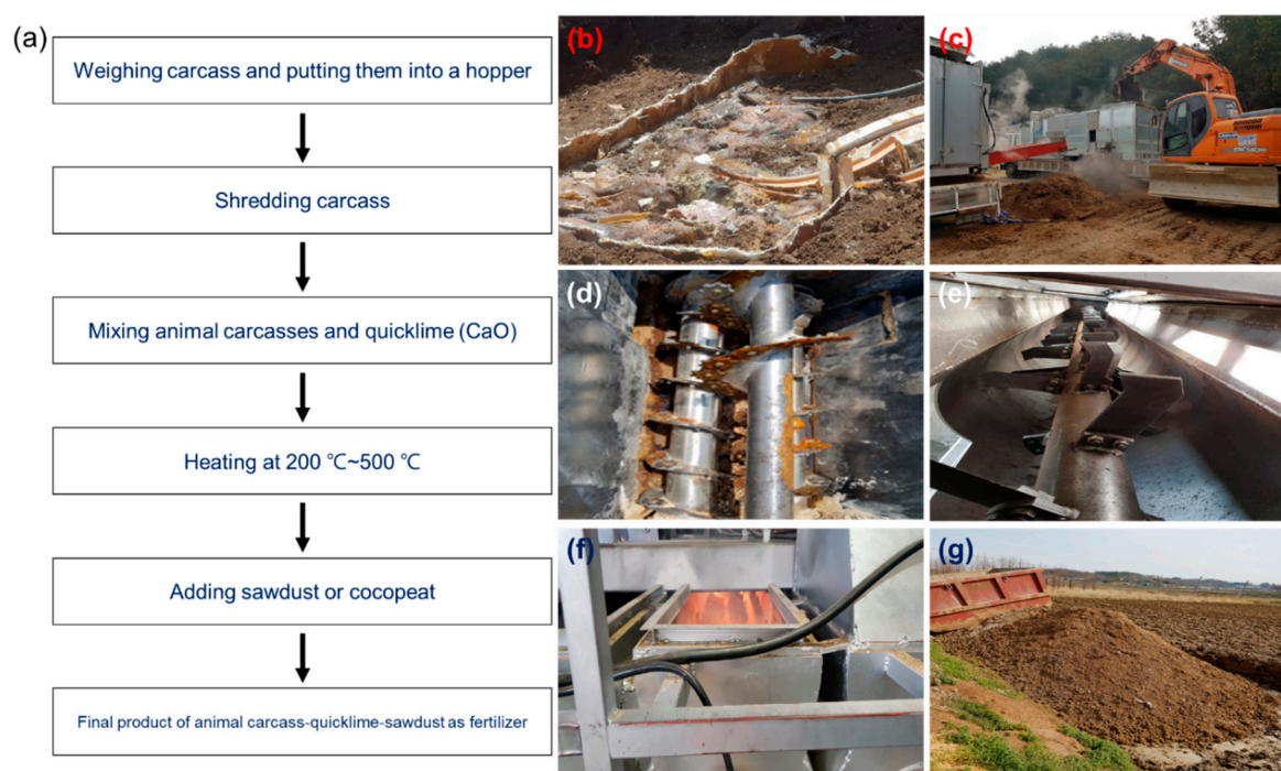
Figure 1. (a) Flow chart of the treatment process in thermo-chemical treatment machinery, (b) animal carcass buried in fiber-reinforced plastic before treatment, (c) placing a carcass into the hopper, (d) shredding carcass, (e) mixing the crushed product with quicklime, (f) heating to 200 °C to 500 °C, (g) final product comprising animal carcass-quicklime-sawdust mixture for use as compost.
