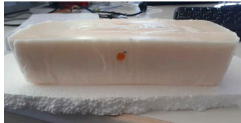
Figure 6. Picture of the produced phantom ( Phantom3 ) used for mm-wave imaging, in which the inclusion is visible.
