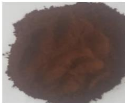
B: Ferrihydrite powder at 75 \mu\text{m}
