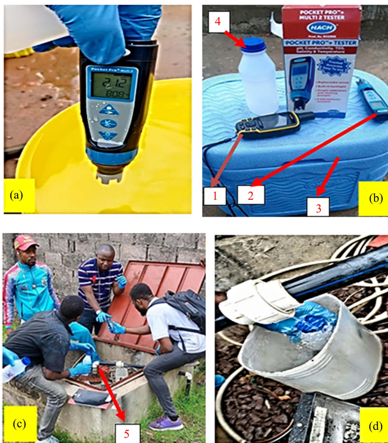
Figure 2. (a): In-situ sampling of pH, T°, TDS, Salinity, electrical conductivity with the multi-parameter probe; (b): Equipment used to collect and preserve samples: a GPS (1), multi-parameter probe (2), a cooler (3), bottle (4); (c): Sampling of the water which leaves the aquifer after pumping before reaching the cistern at the borehole flange level (5); (d): Sampling of water leaving the aquifer after pumping.
