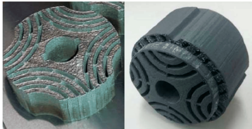
Figure 11. Electric motor core fabricated using L-PBF technique. Reproduced from Reference [86].
