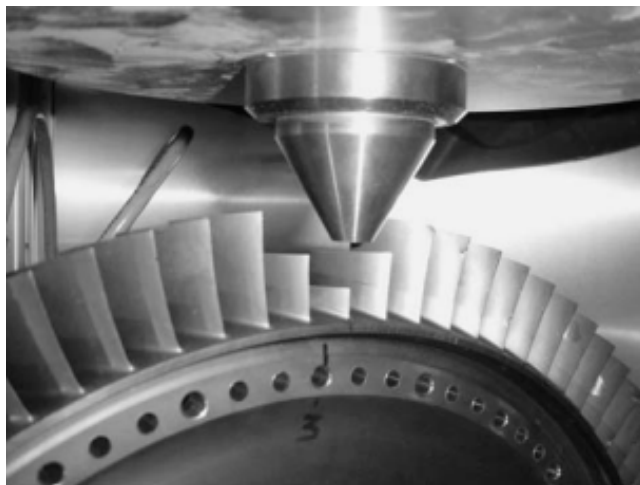
Figure 6. The process of regenerating jet engine rotor blades. Reproduced from Reference [48].
