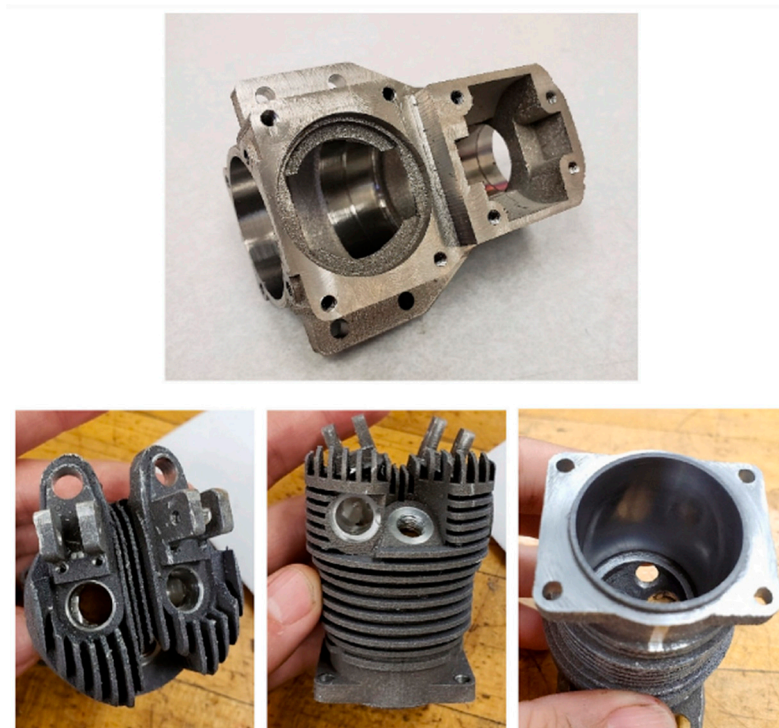
Figure 10. The crankcase ( top ) and the head of the internal combustion engine ( bottom ) of the unmanned ground vehicle. Reproduced from Reference [84].
