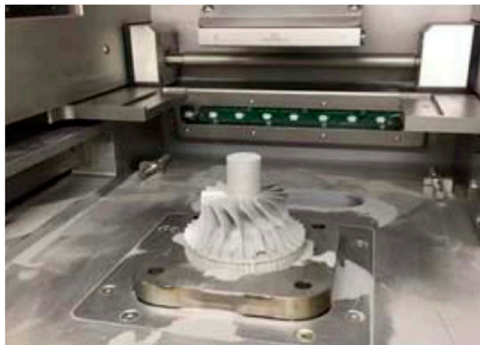
Figure 9. Turbocharger rotor directly after L-PBF process. Reproduced from Reference [80].
