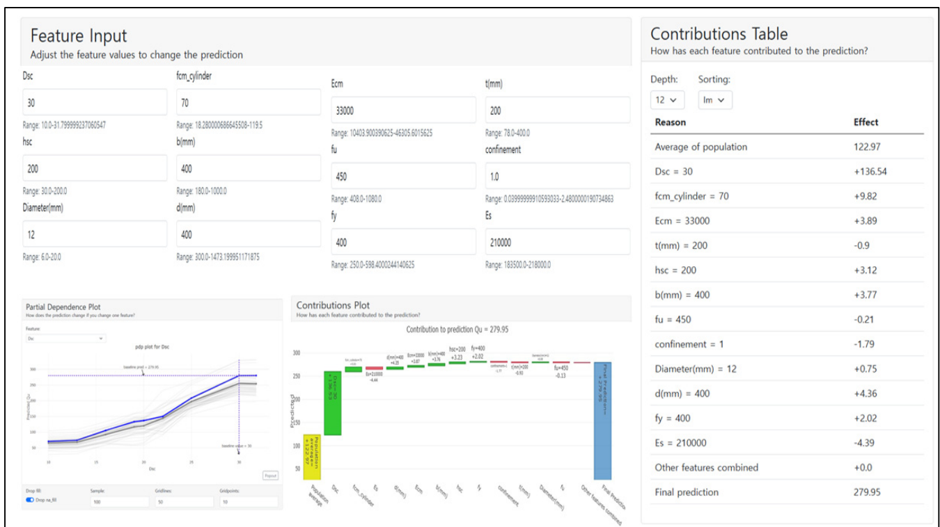
Figure 18. What-if simulation of predictions for the ultimate strength of static shear connections.
