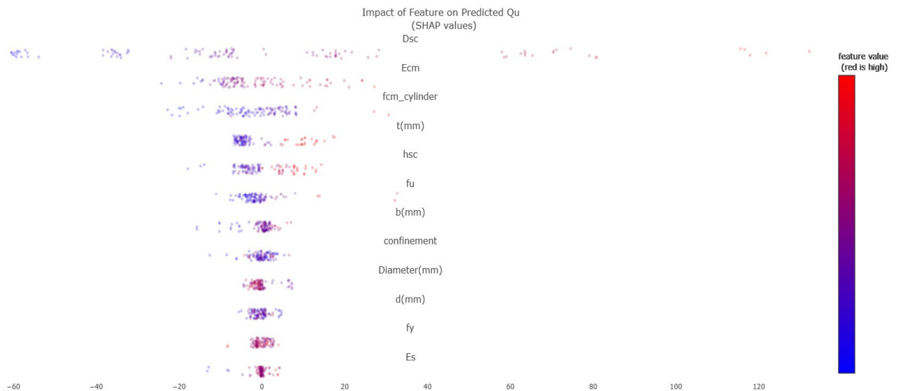
Figure 14. SHAP value of the Voting Regressor for ultimate strength prediction with the augmented dataset.
