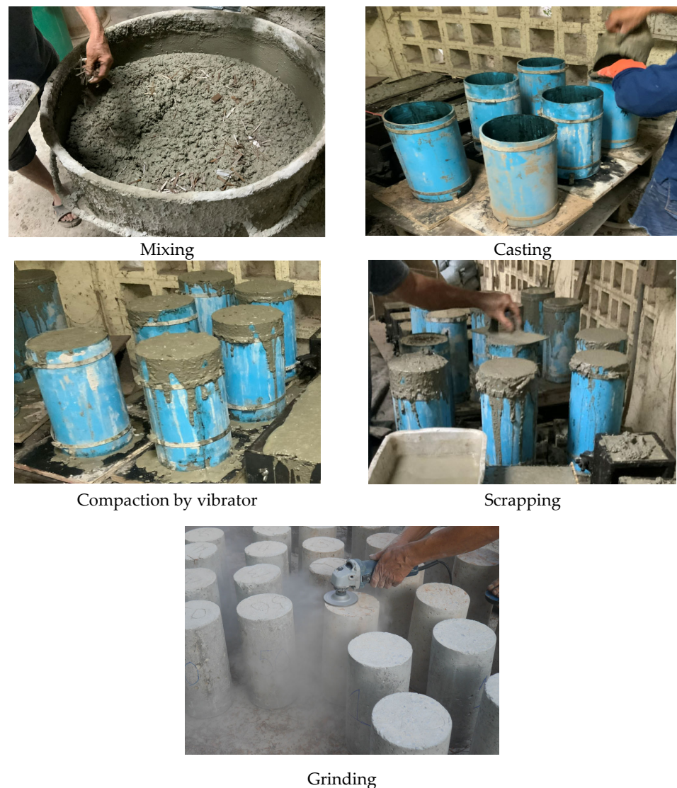
Figure 4. Preparation of test specimens.
