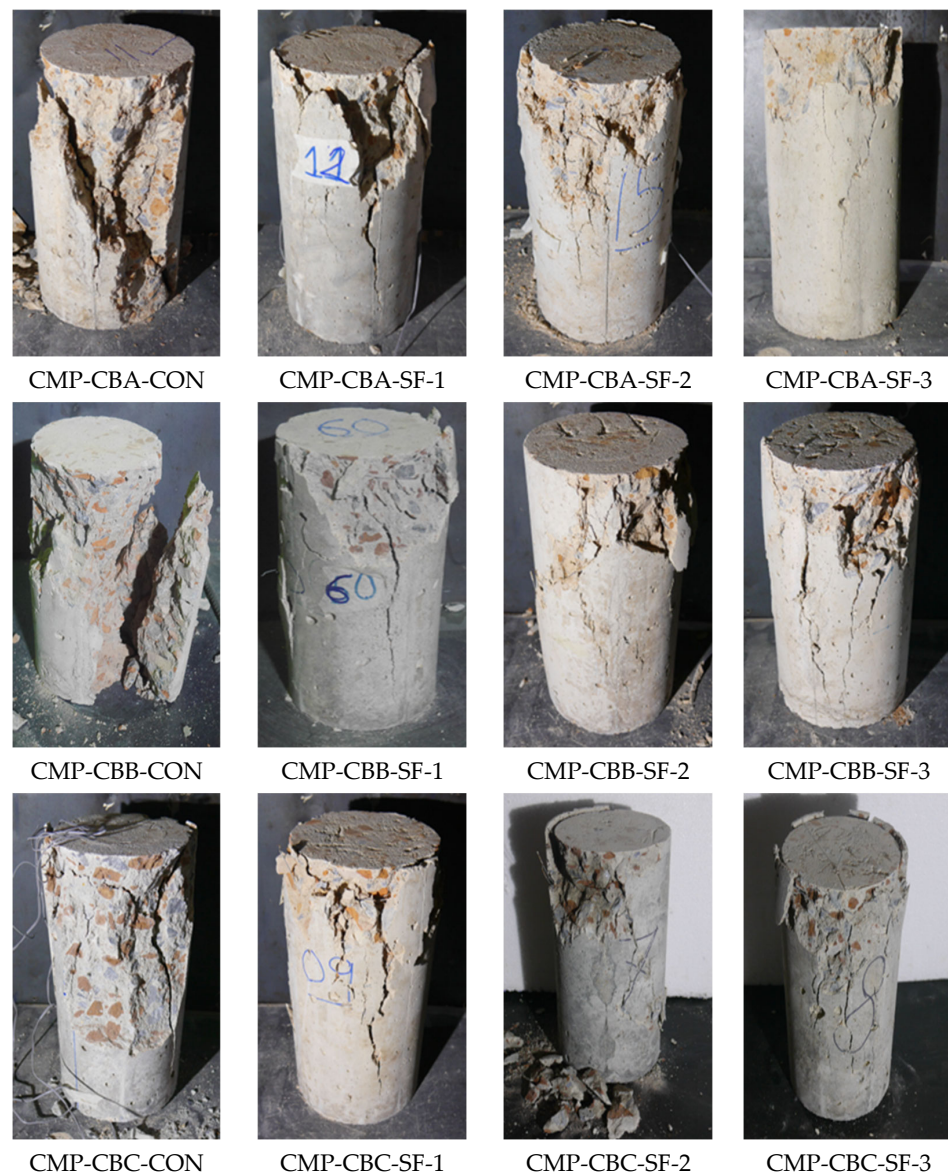
Figure 6. Failure modes observed in all specimens.
