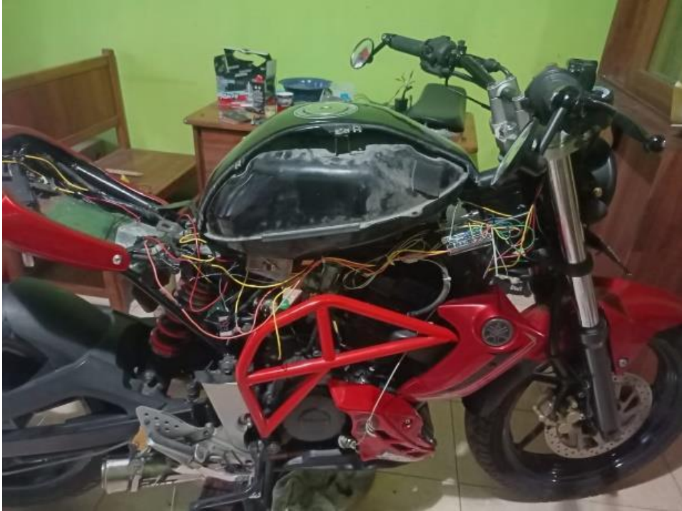
Fig. 7. Elektronik circuit placement
