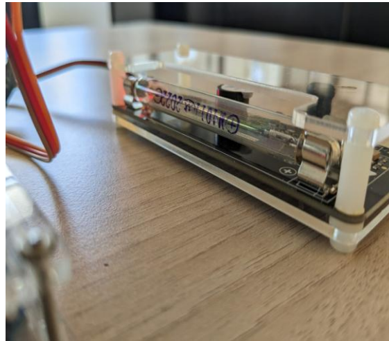
Fig. 3. A Geiger tube with assembled geiger counter circuit
