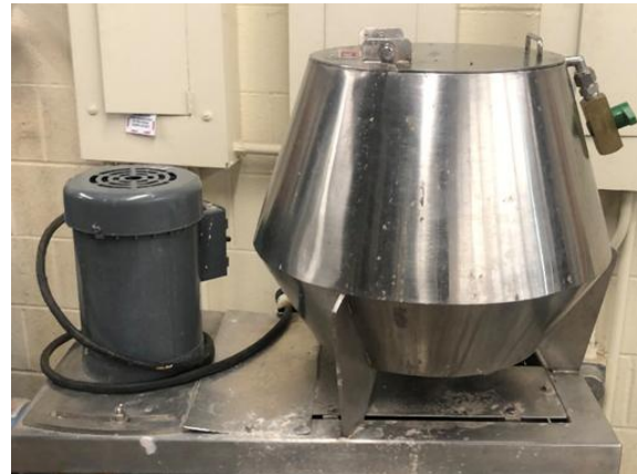
Fig. 2. Low consistency laboratory repulper [1]
