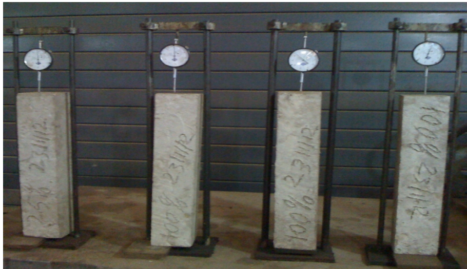
Fig. 1. Loading and measuring frame for shrinkage test
