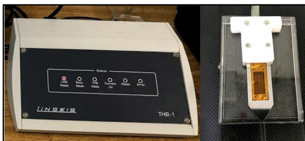
Figure 4. Conductivity meter and THB-1 sensor.
