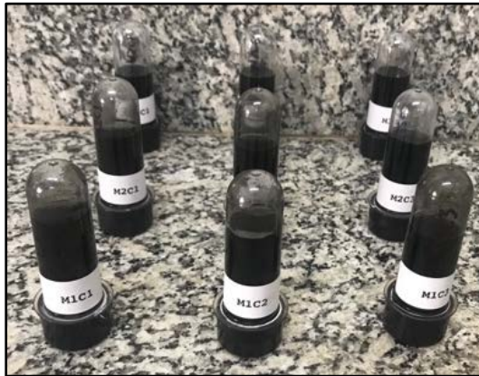
Figure 3. MWCNT/H 2 O nanofluid samples qualitative stability evaluation.
