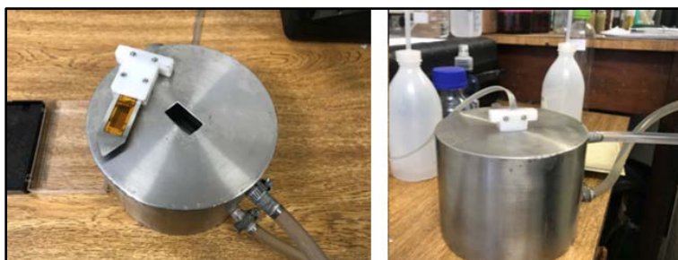
Figure 5. Thermal container and THB-1 sensor.
