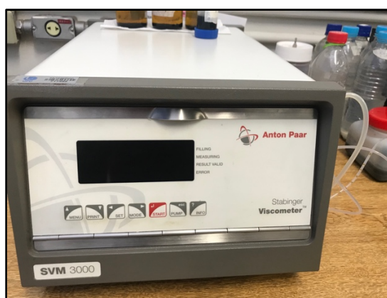
Figure 9. Viscometer used to measure viscosity and density of nanofluid samples.
