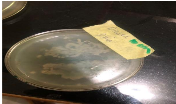
Plate 2. Organisms growing on Minimal Salt Medium supplemented with Diesel as the carbon source
