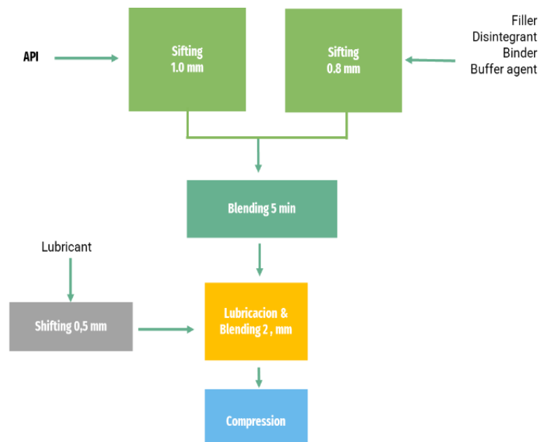
Fig. 3. Manufacturing process flow chart
