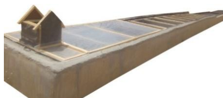
Fig. 1a. Mixed mode on-farm solar dryer Fig. 1b. Indirect mode on-farm solar dryer
