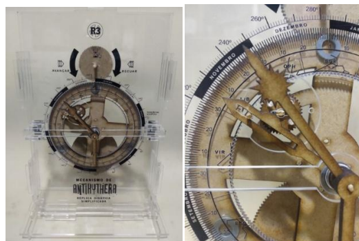
Fig. 7. Replica R3: front face (left) and highlight the epicyclic gear and the planet Mercury pointer (right). Author's design and images
