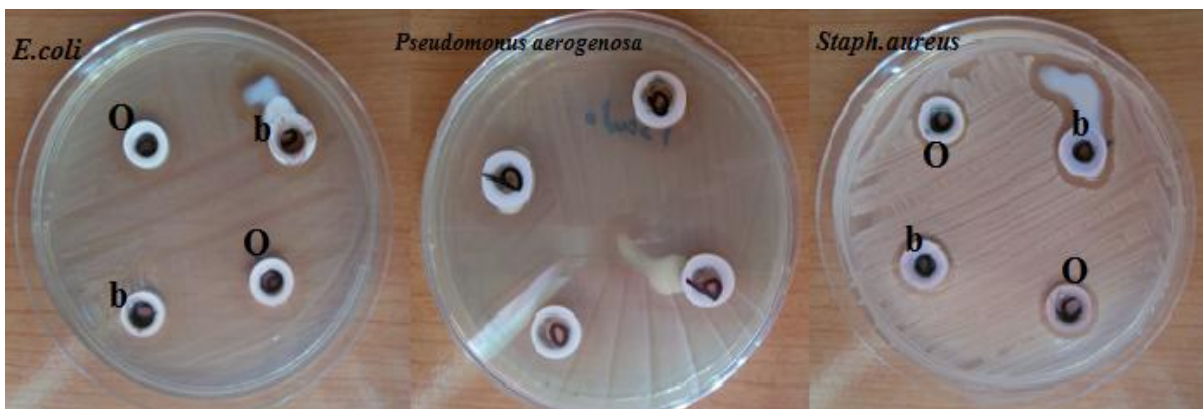
Fig. 6. Inhibition zone of Ag NPs prepared by orange and banana peel extraction on E. coli , Pseudomonas aerogenosa and Staph. aureus bacteria via using good diffusing approaches
