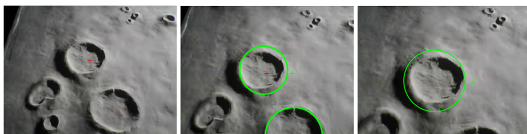
Figure 26. Hazard detection and avoidance procedure for the hardware simulation (images taken at t = 0 s, t = 20 s, and t = 40 s).
