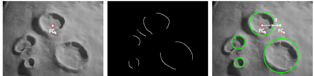
Figure 10. Image acquisition, Canny and circles detection algorithms, and the avoidance approach performed on the lunar terrain of the facility.
