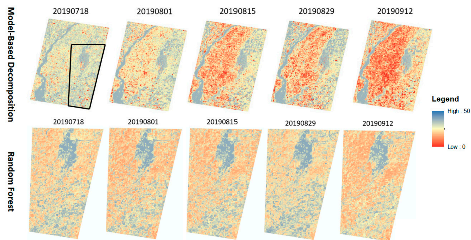
Figure 3. Both the 30 m spatial resolution-derived soil moisture using the two-component model-based decomposition and “zoomed in” (black quadrilateral) example using the random forest machine learning method show the time series trending toward dryer conditions as harvest approaches.
