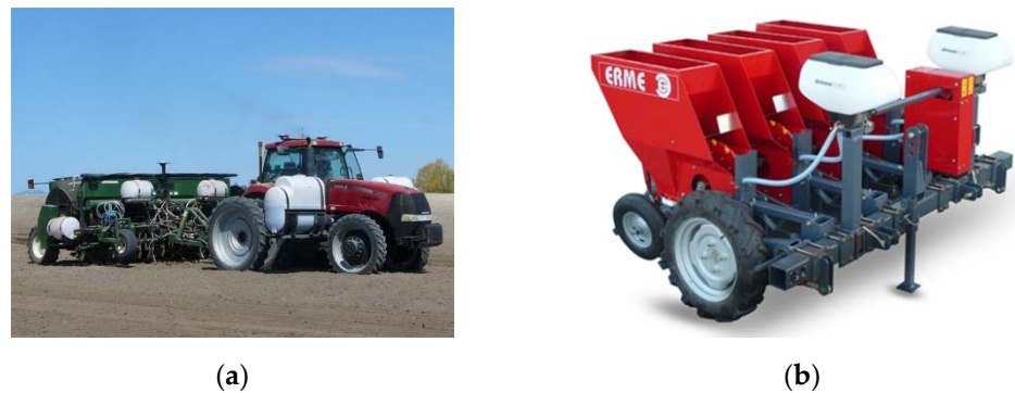
Figure 15. Pneumatic-type potato planter. (a) Lockwood 606. Reprinted with permission from ref. [83]. Copyright 2021 Crary Industries; (b) PLMS 4 rows. Reprinted with permission from ref. [84]. Copyright 2020 Engineering & Manufacturing Aircraft Tools.
