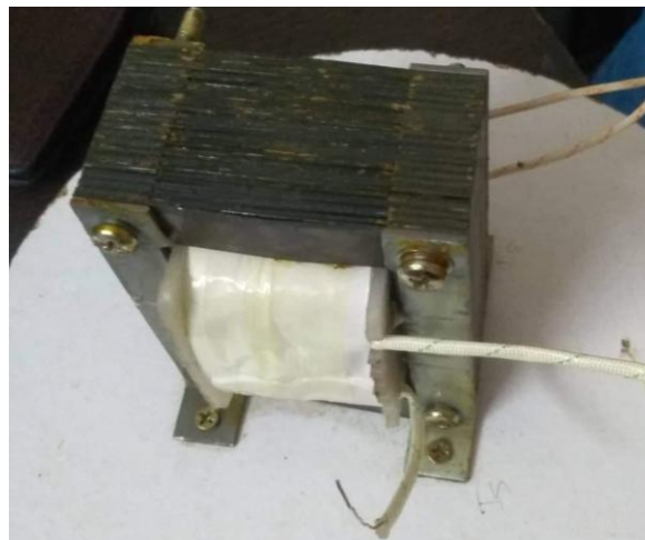
Fig. 5. Manufactured single-phase transformer on the base
