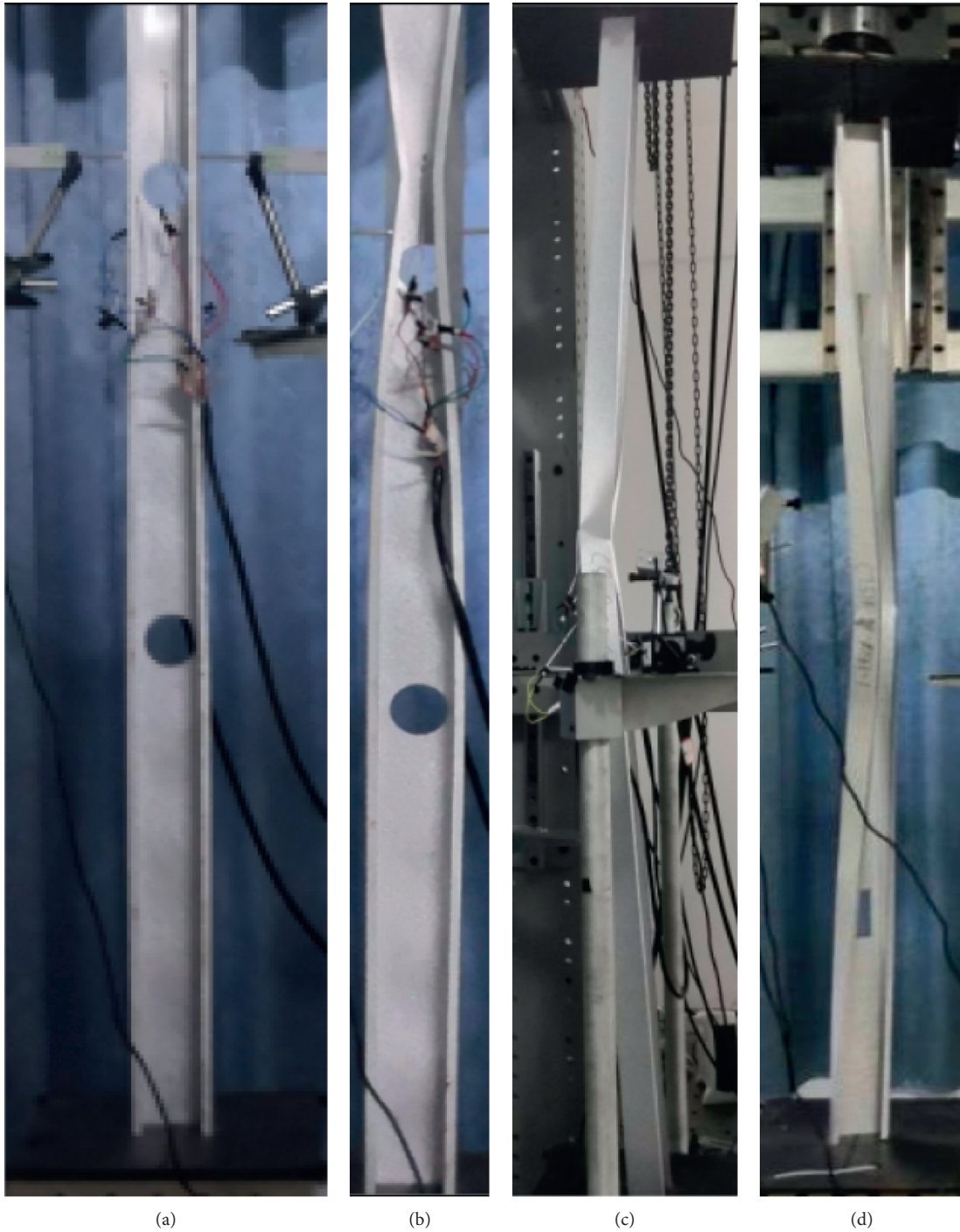
FIGURE 11: Buckling modes of specimens with a length of 2000 mm. (a) Local buckling. (b) Distortional buckling. (c) Flexural buckling. (d) Flexural-torsional buckling.
