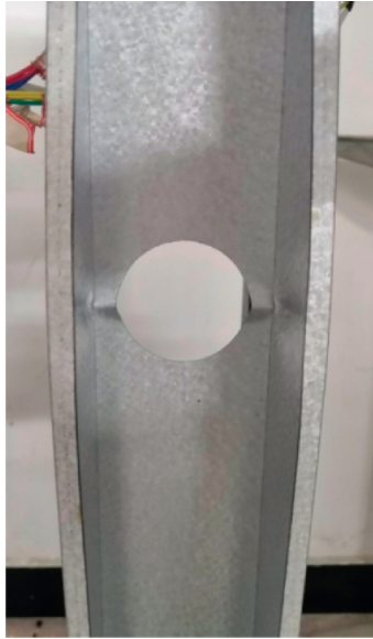
FIGURE 12: Plastic local buckling failure of plates adjacent to holes.
