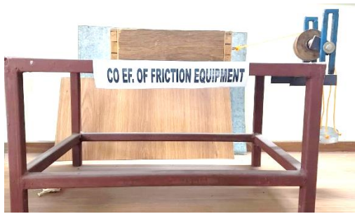
Fig. 4. Measurement of coefficient of friction w.r.t. different materials
