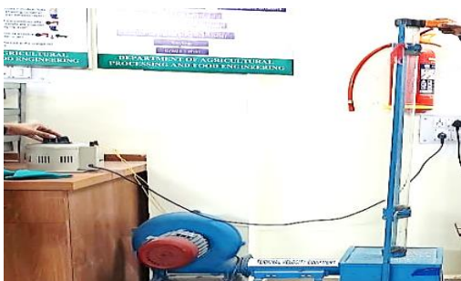
Fig. 5. Measurement of terminal velocity
