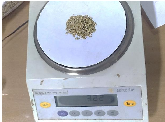
Fig. 2. Measurement of 1000 grain weight
