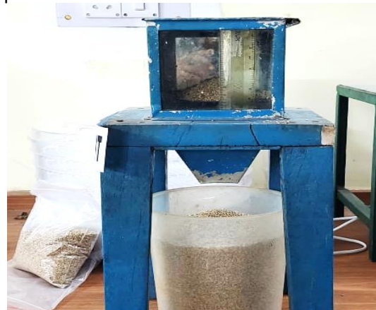
Fig. 3. Measurement of angle of repose
