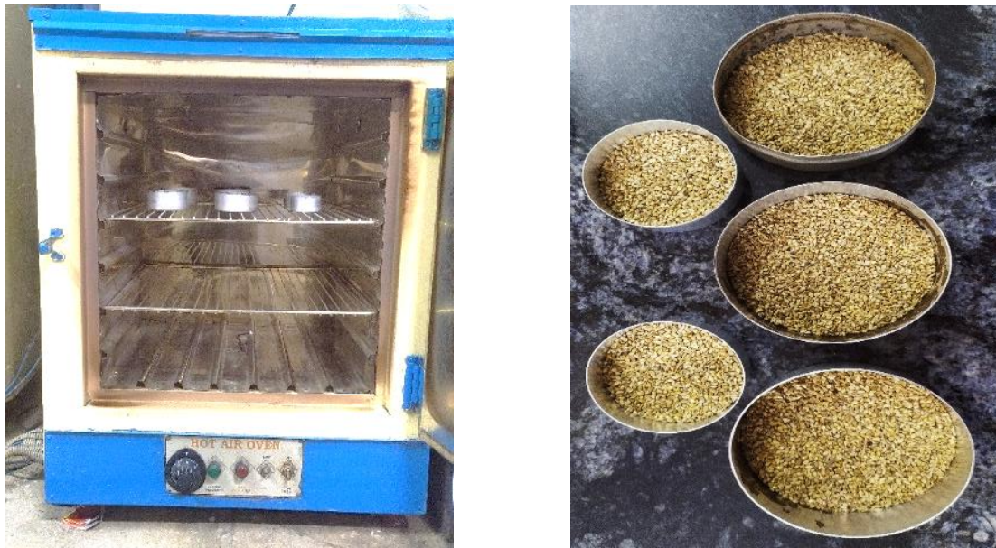
Fig. 1. Measurement of moisture content through oven drying
