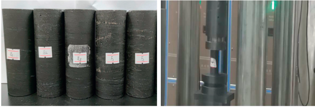
FIGURE 10: WAW31000 microcomputer-controlled electrohydraulic servo testing machine.
