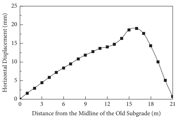
FIGURE 8: Horizontal displacement of subgrade top surface.
