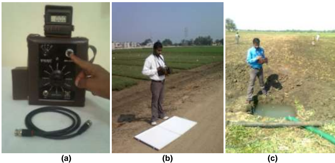
Fig. 3. Measurement of reflected energy ( W/cm^2 Sr-micron), (a) Ground truth radiometer (GTR), (b) Total energy Calibration plate ( BaSO_4 ), (c) Observation on object
