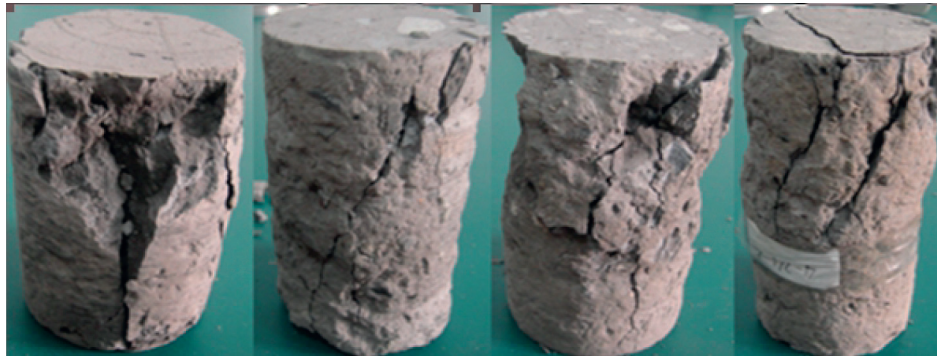
FIGURE 9: Photograph of broken filling paste after uniaxial compression test.
