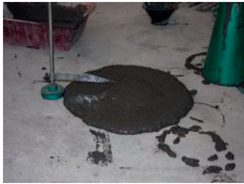
FIGURE 2: Slump meter test.
