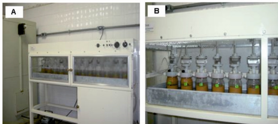
Fig. 1. Multi-cell bioreactor system used in the bioremediation tests: A) Front view of the equipment; B) interior view showing the air-feed tubes and the mechanism of rotation of the flasks
