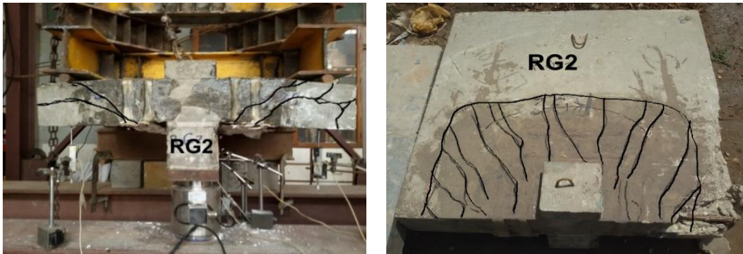
Fig. 32. Cracking pattern of specimen (RG2)
