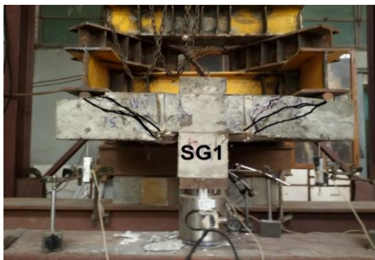
Fig. 23. Cracking pattern of specimen (SG1)
