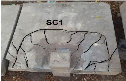
Fig. 24. Cracking pattern of specimen (SC1)
