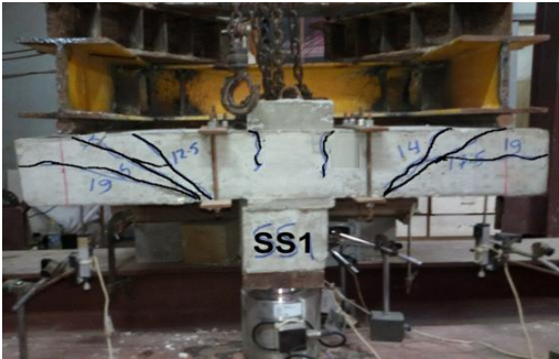
Fig. 25. Cracking pattern of specimen (SS1)
