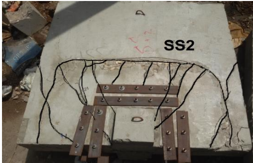
Fig. 28. Cracking pattern of specimen (SS2)
