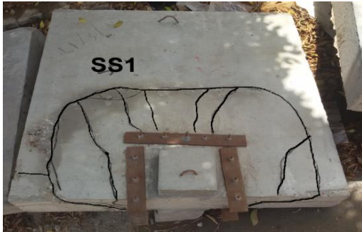
Fig. 25. Cracking pattern of specimen (SS1)
