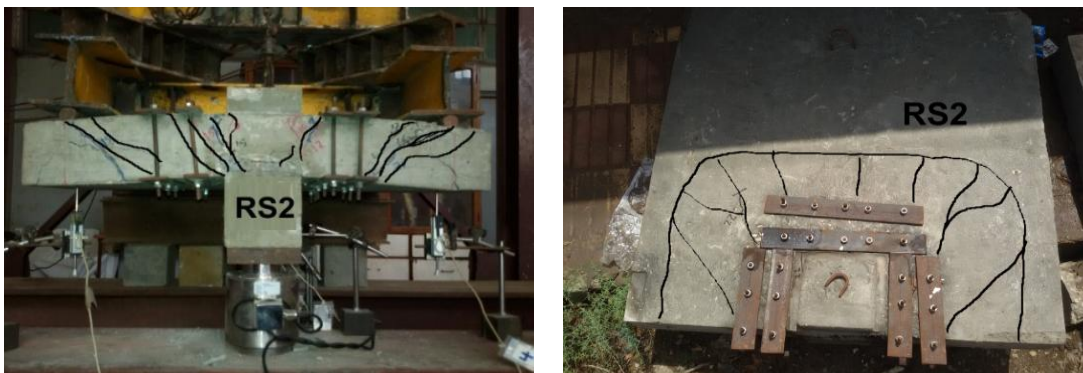
Fig. 34. Cracking pattern of specimen (RS2)
