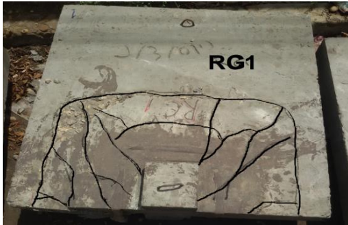
Fig. 29. Cracking pattern of specimen (RG1)
