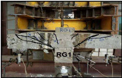
Fig. 29. Cracking pattern of specimen (RG1)
