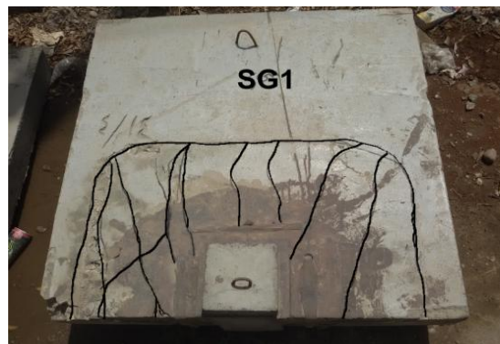
Fig. 23. Cracking pattern of specimen (SG1)
