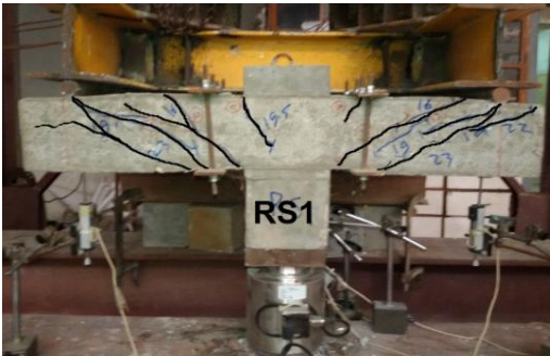
Fig. 31. Cracking pattern of specimen (RS1)
