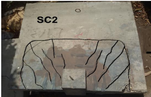
Fig. 27. Cracking pattern of specimen (SC2)
