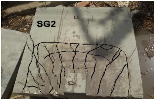
Fig. 26. Cracking pattern of specimen (SG2)
