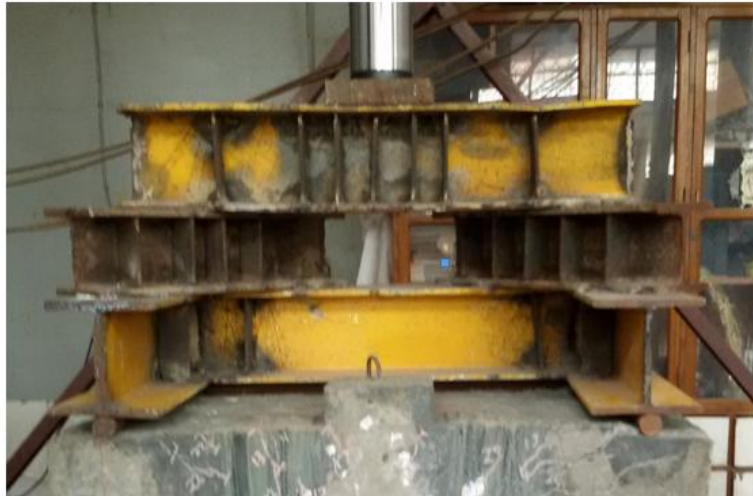
Fig. 7. The rigid steel system used to distribute the concentrated load
