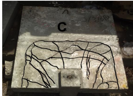
Fig. 22. Cracking pattern of specimen (C)
