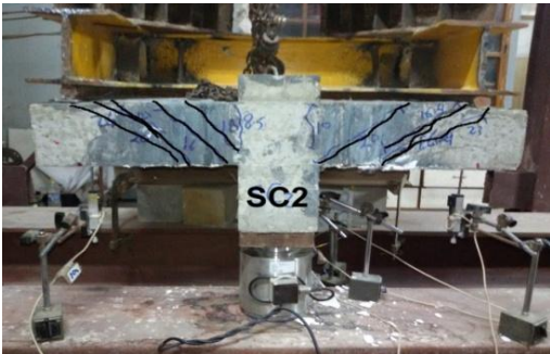
Fig. 27. Cracking pattern of specimen (SC2)
