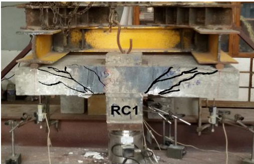
Fig. 30. Cracking pattern of specimen (RC1)
