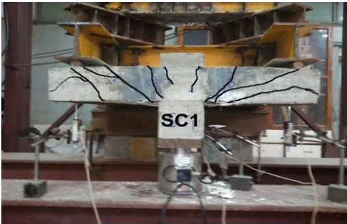
Fig. 24. Cracking pattern of specimen (SC1)
