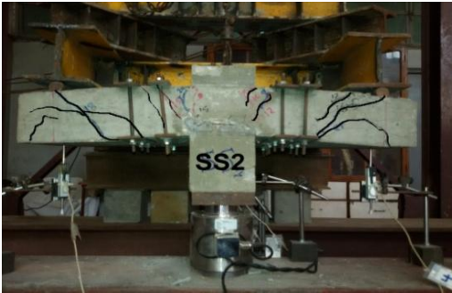
Fig. 28. Cracking pattern of specimen (SS2)
