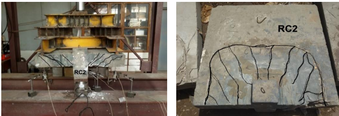
Fig. 33. Cracking pattern of specimen (RC2)
