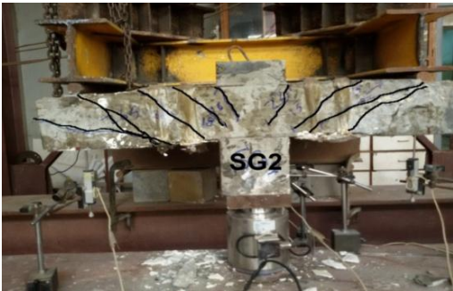
Fig. 26. Cracking pattern of specimen (SG2)
