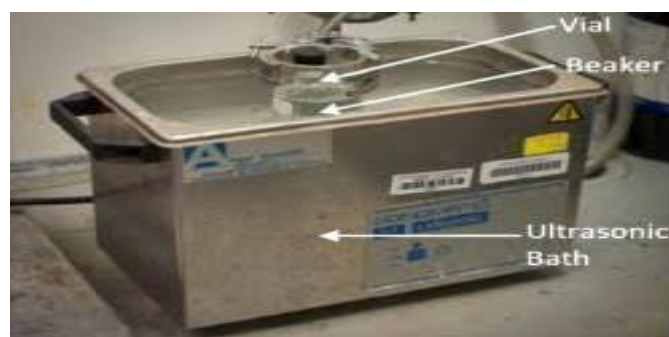
Fig. 6. Showing diagrammatic instrumentation of the Sonication bath ( https://www.sciencedirect.com/topic/chemistry/sonication )
