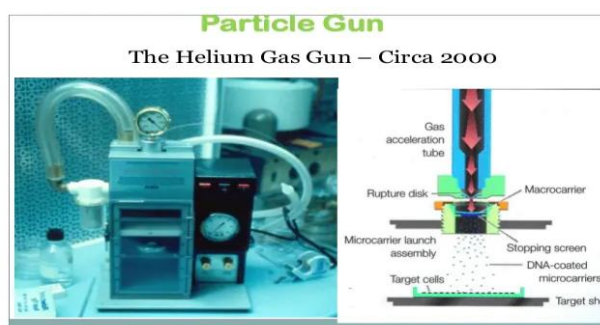
Fig. 2. Showing the instrumentation of particle bombardment method of plant transformation technique ( https://slidetodoc.com/direct-dna-transfer-introduce-dna-into-cells-assay/ )
