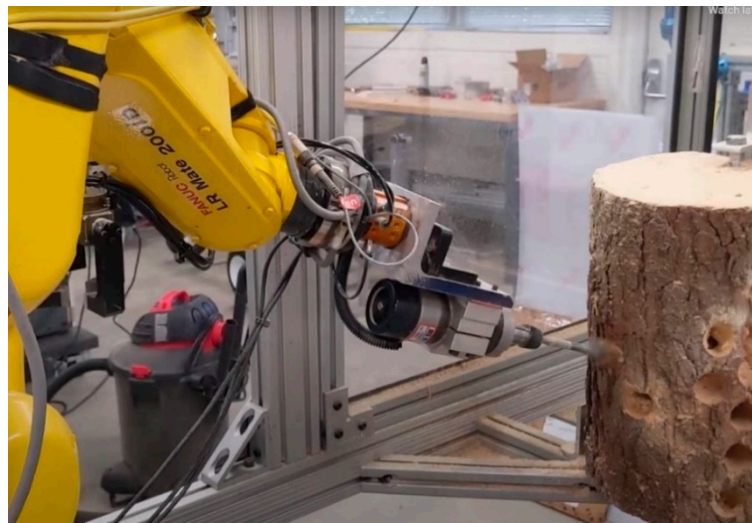
Figure 4. Drilling tool during a borehole drilling operation.
