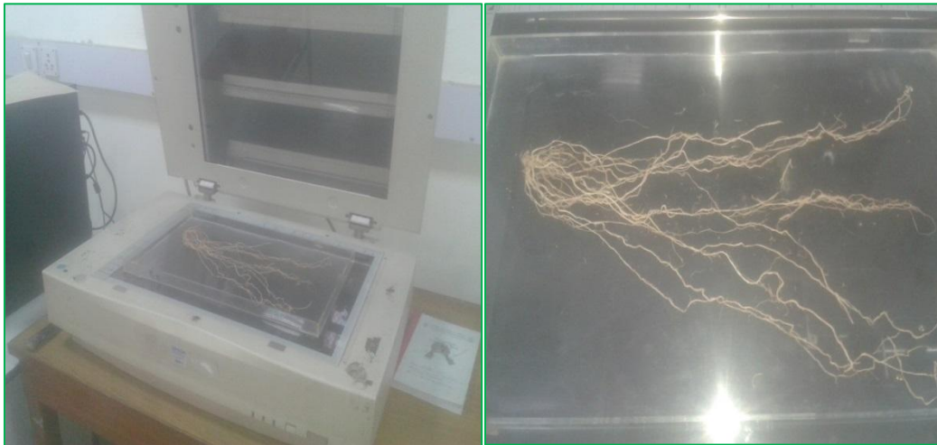
Fig. 1. Scanning of maize root in Win RHIZO root scanner
