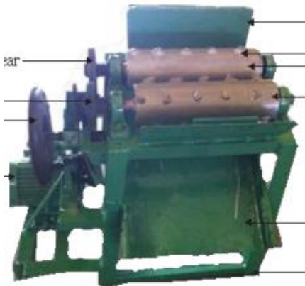
Fig. 1.16. Coconut dehusking machine with flywheel
