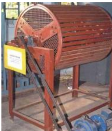
Fig. 2.3. CPCRI batch type coconut deshelling machine
