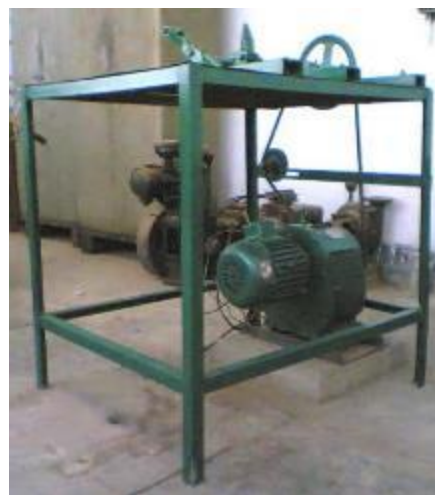
Fig. 1.4. Cam and follower type coconut dehusker
