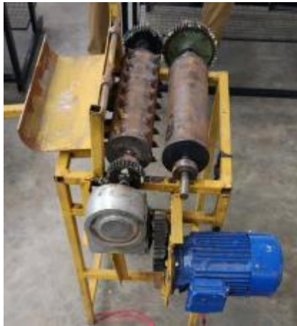
Fig. 1.14. Single spiked roll type coconut dehusking machine
