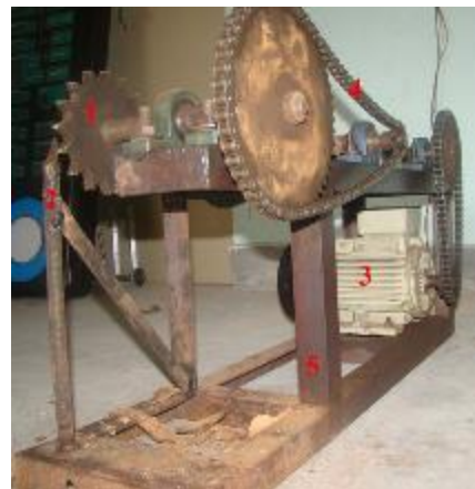
Fig. 2.2. Coconut deshelling machine (Belt and pulley drive)
