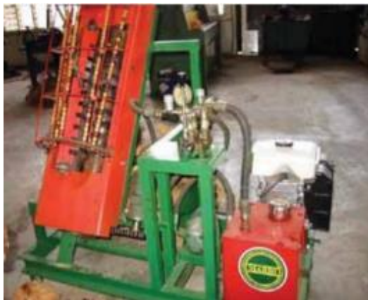
Fig. 1.10. Petrol engine powered coconut dehusking machine
